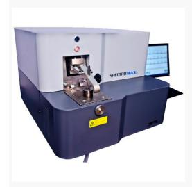
The SPECTRO MAXx stationary metal analyzer is used mainly for material testing in foundries and for incoming and outgoing inspections in the metal industry around the world. It determines all of the elements used in the metal industry, including metal analysis of carbon, phosphorous, sulfur and nitrogen.
